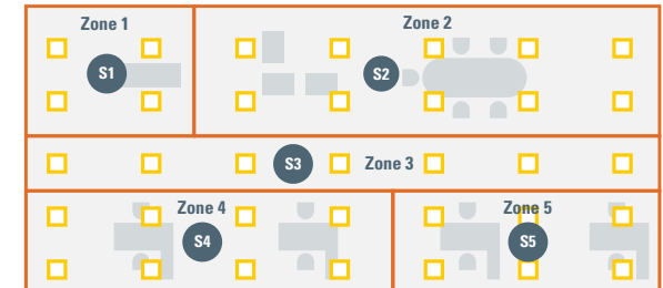
Figure 17 Sensors are Mounted External to Luminaires in Zone-Based Control
